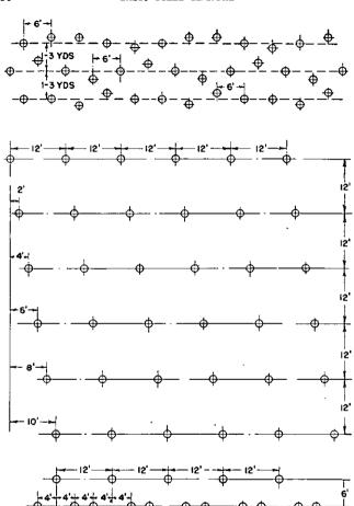
Figure 20.—Methods of arranging band of antitank mines.
